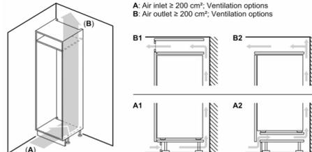
A: Air inlet  $\geq 200 \text{ cm}^2$ ; Ventilation options
